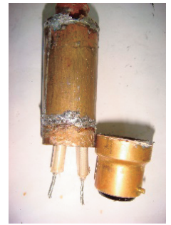
photo app.1-11 Electric wire state in socket
