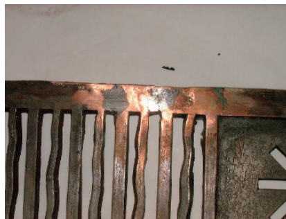
photo app.2-16 Damaged frame attachment
