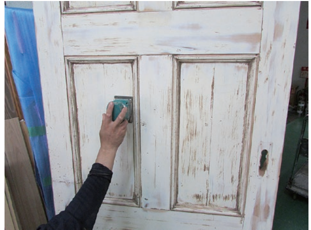
photo 14 Graining process ① sander scraping
