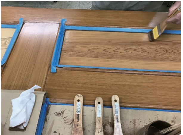
photo 22 Graining process (medium figured grain) ⑥ -5 panel board straight grain brush pulling
