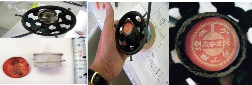
photo app.1-57 Light-blocking plug (with no light bulb fitted in the socket)
