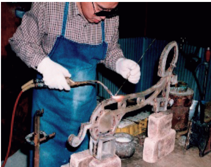
photo 67 Welding the arm
