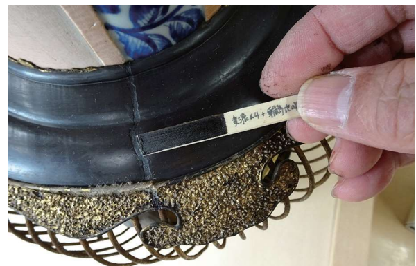
Fig. 16 Color adjustment of the crack — comparing the color with the sample board.
