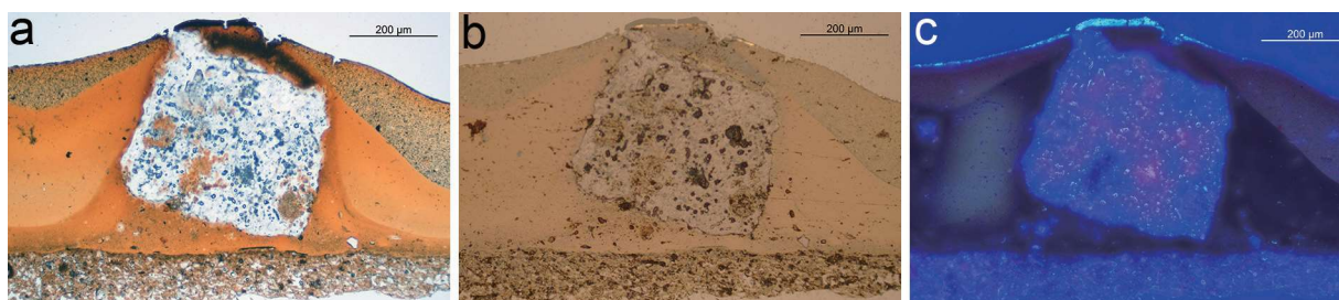
Fig. 6 Cross-section of the protrusion part. a: transmission image. b: reflected image. c: UV image.
