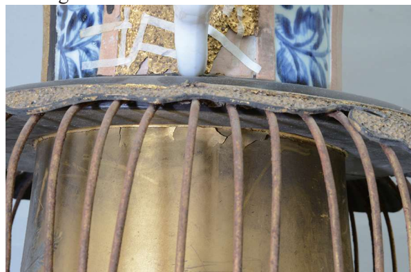
Fig. 2 The condition of gold leaf applied to Urushi and iron bar.
