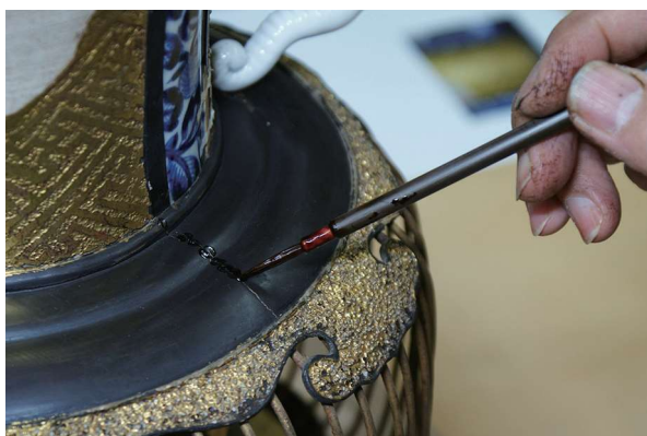
Fig.7 Urushi served as a main component for many restoration steps. The image shows filling a crack with diluted mugi-urushi .
