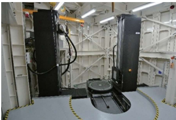
Fig.2 X-Ray CT scanner used in this project: The world's largest-class CT for cultural property that scans the object in the maximum DIA. 2.5 m, H. 2.5 m, WT. 500 kg without moving it from the carriage. X-ray tube: 600 kV (strong enough to take the tomographic image of 80 mm. pure iron).
