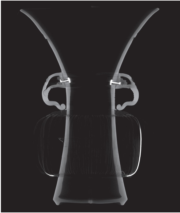
Fig. 9 Vertical tomographic image around the centre of the vase.
