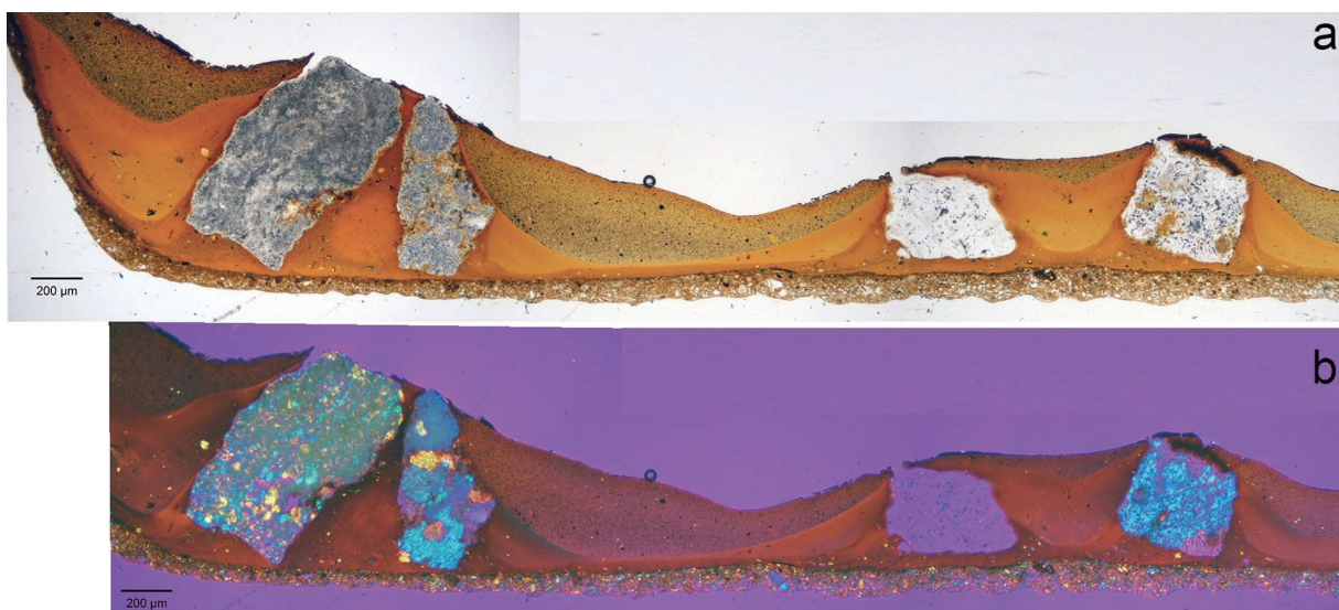
Fig. 5 Cross section image of the protrusion part. a: transmission image. b: polarized image.
