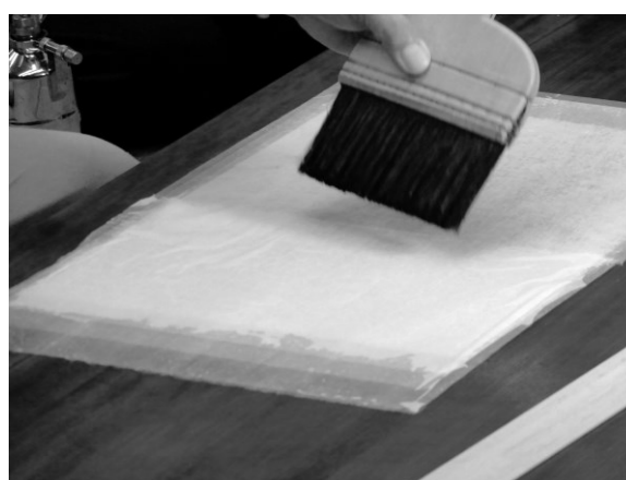
Fig. 29 Smooth the surface well with a nadebake 撫で刷毛で表面をよく撫でる
