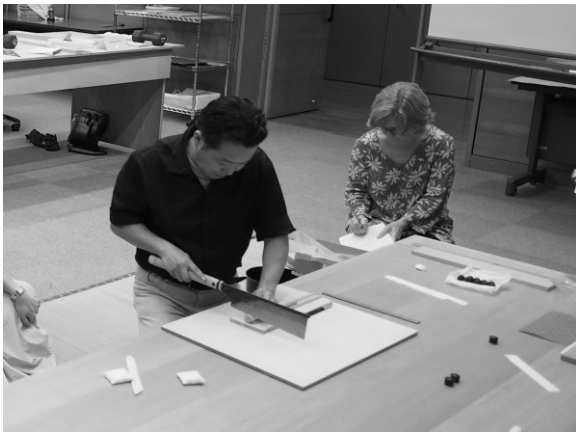
Fig. 52 Cut the roller rod in calculated length 軸を算出した長さで切る
