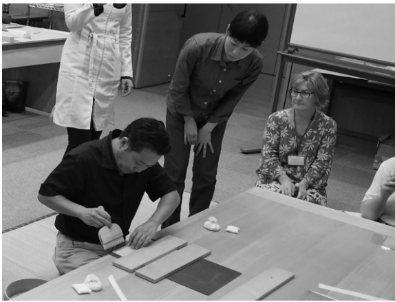
Fig. 50 Attach the head rod to the cover with paste 表紙に八双を糊でつける
