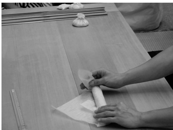
Fig. 74 Fold both corners of paper inside 両端の紙を内側に折り込む
