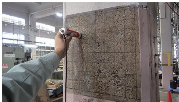
photo 7-8: Spontaneous potential measurement (photo provided by : West Japan Railway Company)
