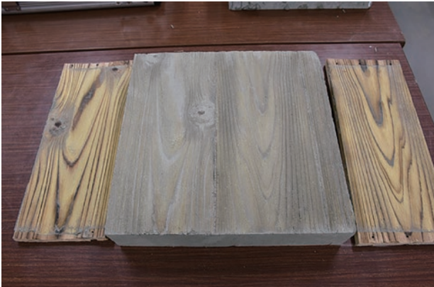
photo 5-11: Surface roughening (embossing) made on a trial basis (photo provided by : The Japanese Association for Conservation of Architectural Monuments)
