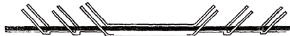
figure 4 Kahn style reinforcement for beams. Although the diagonal reinforcement is said to have been designed to bear shear force, it does not appear effective. (Source: 日比忠彦、鐵筋混凝土ノ理論及其應用 上卷、丸善株式会社、1916.1 初版、photo provided by: Japan Society of Civil Engineers, JSCE Library、 http://library.jsce.or.jp/Image_DB/s_book/jsce100/pdf/20612/20612_03.pdf 、p.315)
