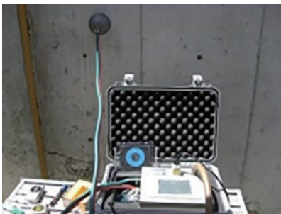
photo 7 Air-permeability test of the concrete covering the rebar
