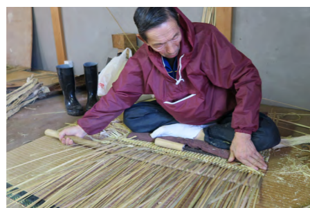
ヒゴの間にフジを叩きこむ(富山 論田熊無の箕) Japanese wisteria is inserted between the splits and tapped in place.
