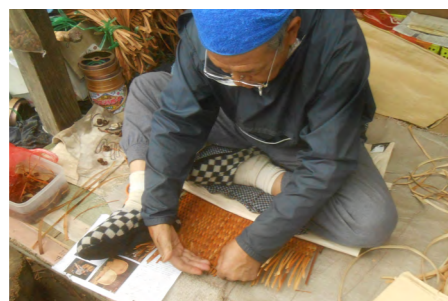
北東北では道具を使わずで材を押し込むところが多い(岩手 面岸の箕) In many places in northern Tohoku, the material is pushed in by hand without using any tool.
