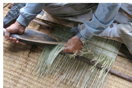
上下のヒゴの間をミガタナで開く(鹿児島 日置箕) The space between alternately raised and lowered splits of materials is opened wide using a mi-gatana .
