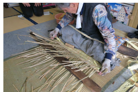
開いた織り口をナギナタで押さえておく(長野 戸隠箕) The open weaving end is held down with a naginata .
