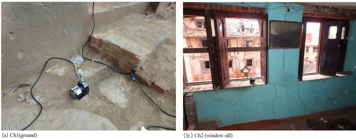
Fig. 3-3-6 Velocity-meters
