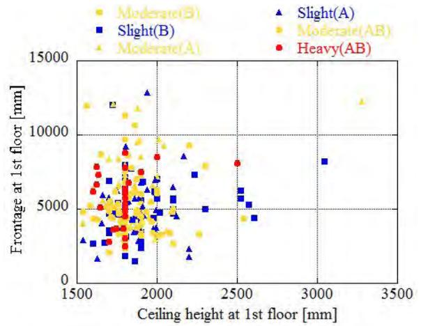
Fig. 3-2-8 Relation between the ceiling height, the frontage at first floor, and degree of damage
