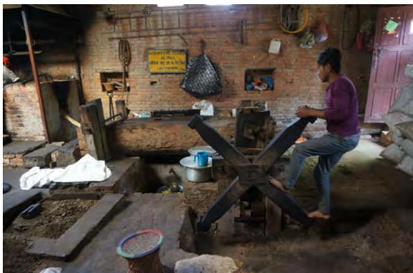
Fig. 2-3-8 The way of compressing using the weight of the workman
