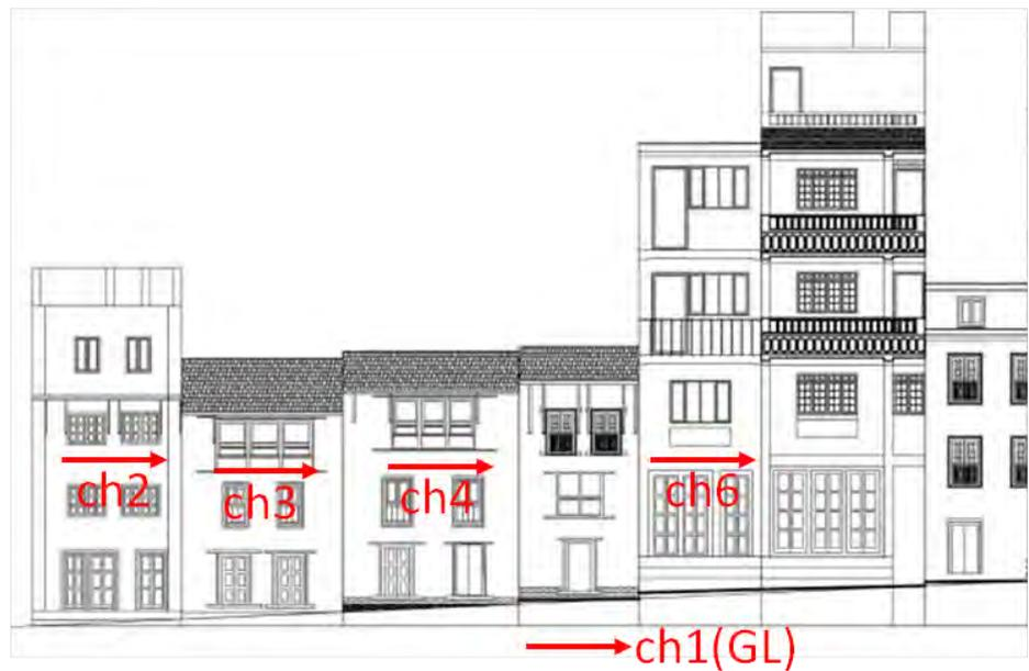
Fig. 3-3-4 The measurement points which velocity-meters are placed
