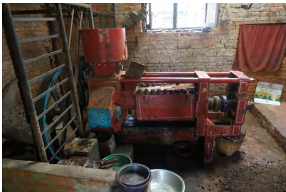
Fig. 2-3-9 Mechanical compressor used for second squeeze
