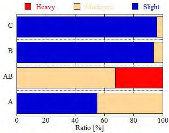
Fig. 3-2-1 Relation between the type of building structure and degree of damage
