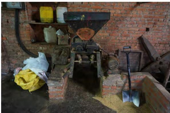
Fig. 2-3-6 The grinding mill for mustard seeds
