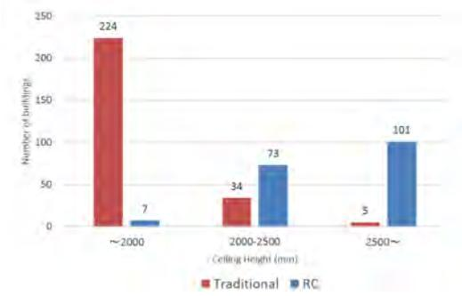
Fig. 3-1-13 Ground floor ceiling height of traditional and non-traditional buildings
