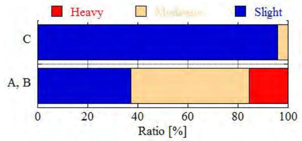
Fig. 3-2-2 Relation between the type of building structure and degree of damage (Type A and B is combined)
