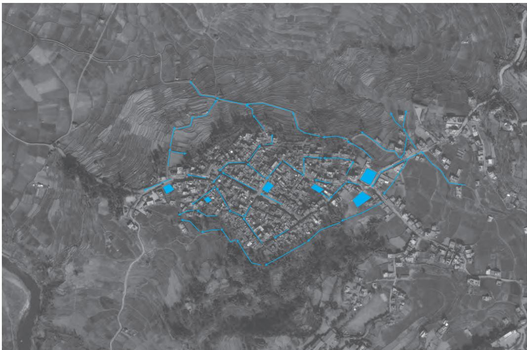
Fig. 2-7-2 Inside of Khokana village and its surrounding irrigation and drainage system
