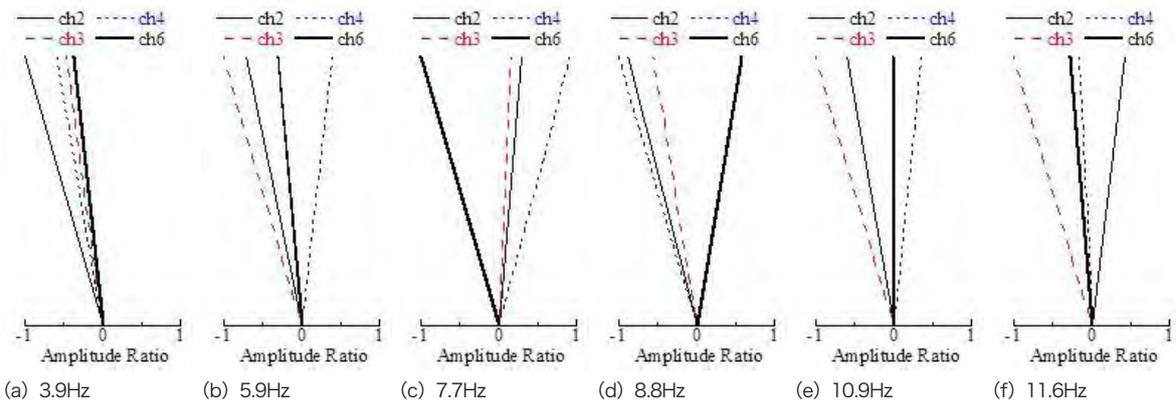
Fig. 3-3-8 Vibration mode (case 2)
