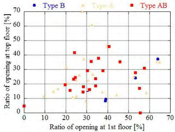
Fig. 3-2-14 Relation between the ratio of opening at first floor and that at top floor
