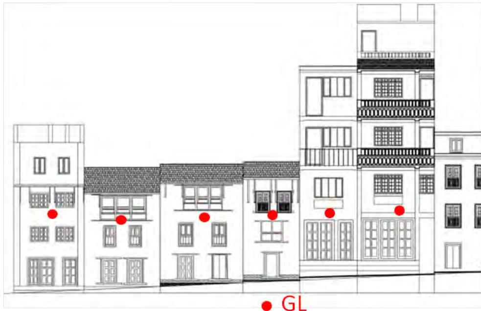
Fig. 3-3-2 The measurement points which velocity-meters are placed
