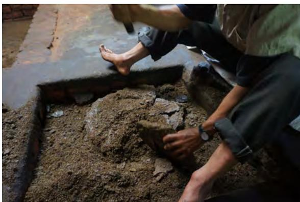
Fig. 2-3-13 Crushing pomace of first squeeze
