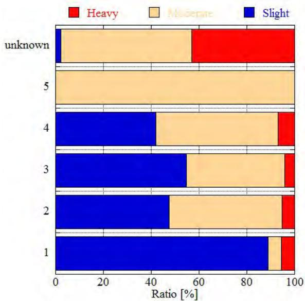
Fig. 3-2-5 Relation between the number of building story and degree of damage
