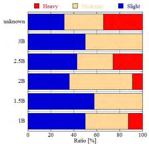
Fig. 3-2-6 Relation between the thickness of the walls at the first floor and degree of damage
