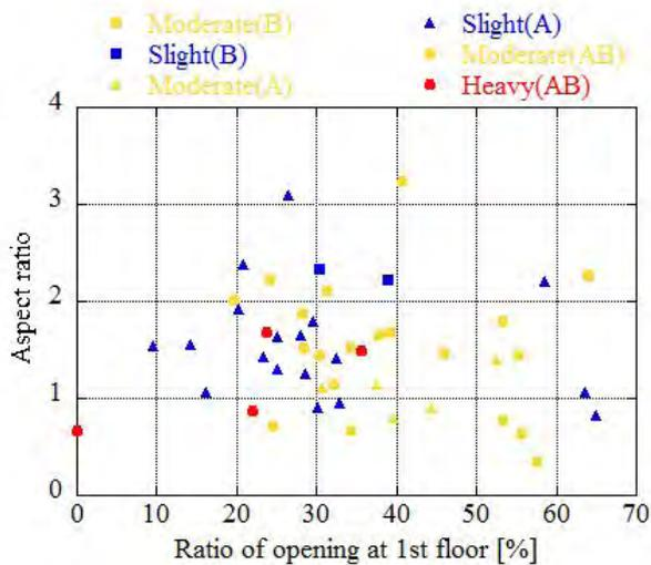
Fig. 3-2-15 Relation between ratio of opening and aspect ratio at first floor
