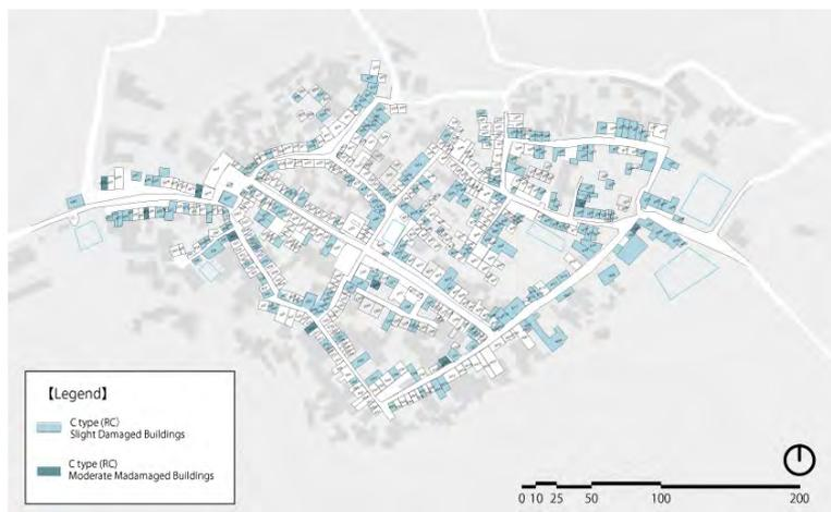
Fig. 3-1-9 Distribution map of non-traditionally constructed buildings in southern settlement area (Slight and moderate damage)
