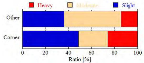
Fig. 3-2-4 Relation between the position of the buildings and degree of damage
