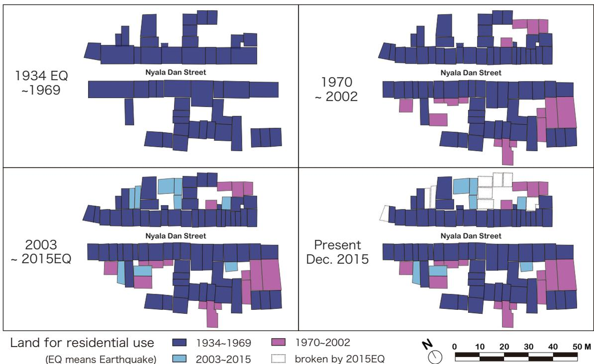
Fig. 2-6-46 Transition of courtyards with extension of housings
