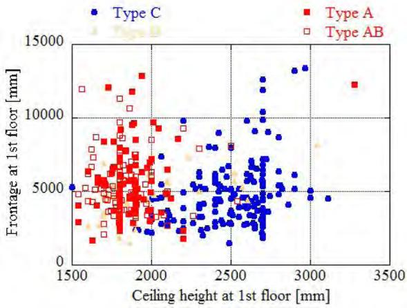
Fig. 3-2-7 Relation between the ceiling height and the frontage at first floor
