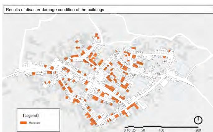
Fig. 3-1-7 Distribution map of half-collapsed traditionally constructed buildings in the southern settlement area
