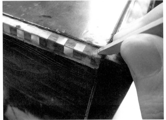
Fig. 9.15 刻苧の調整 Adjusting the kokuso surface
