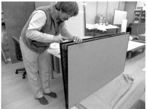
(12) 金物取り付け Affixing the metal fittings
