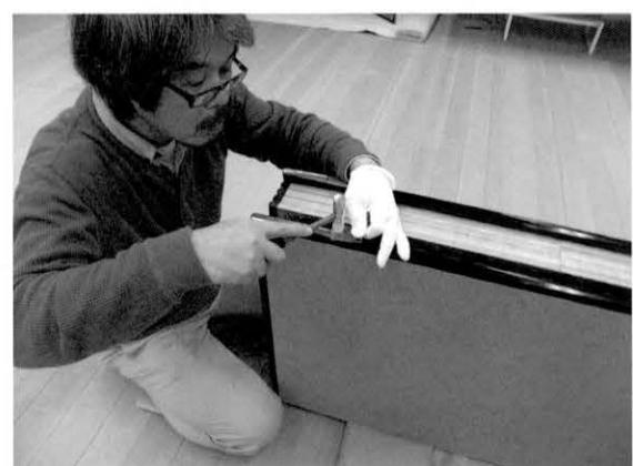
(6) 仕上げ(飾金物取り付け) Finishing (attaching the metal ornaments)
