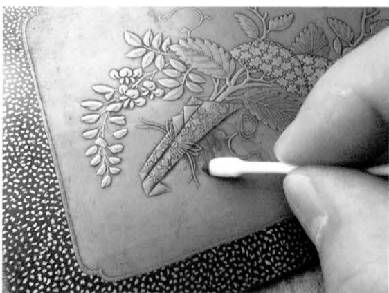
図15 塗料除去 Fig. 15 Removing the coating material
