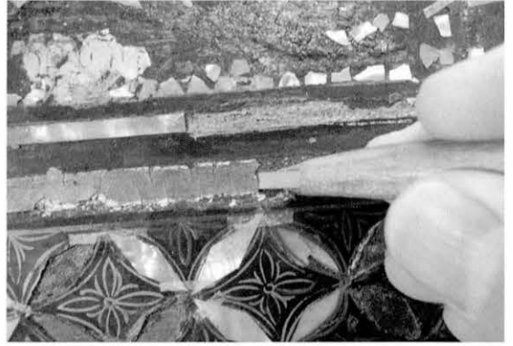
後補充填の除去 Removing filler from past restorations
