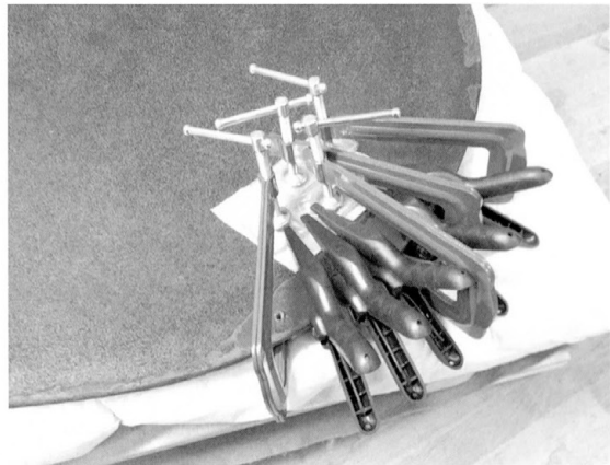
図20 膠含浸後 クランプ圧着 Fig. 20 After impregnating animal glue, press-stabilizing with clamps
