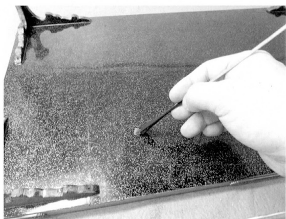
図33 裏面 漆固め Fig. 33 Underside, consolidation
