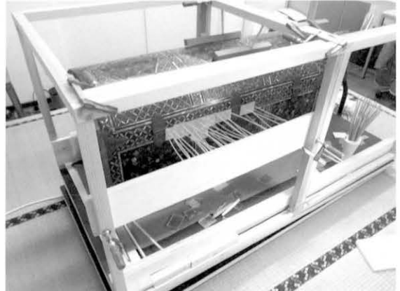
図16 木枠内での芯張り圧着 Fig.16 Press-stabilizing in a wooden shimbari frame
