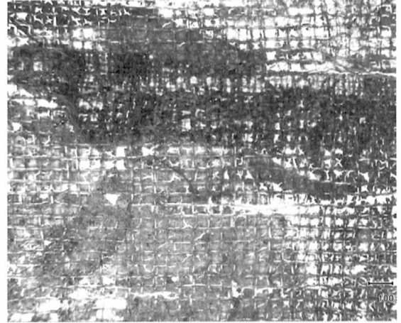
図4 旧補絹：②細かい目・太い糸 Fig. 4 Old mending silk : fine weave, thick thread (type ②)
