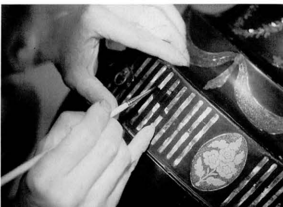
94 膠の含浸 Impregnating animal glue under the shell pieces
