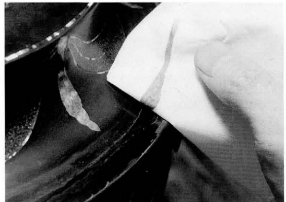
100 蒔地の固め Consolidating the diatomaceous earth
