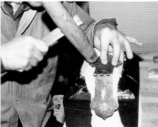
図114 錠金具の形状修正 Reshaping the metal fitting
