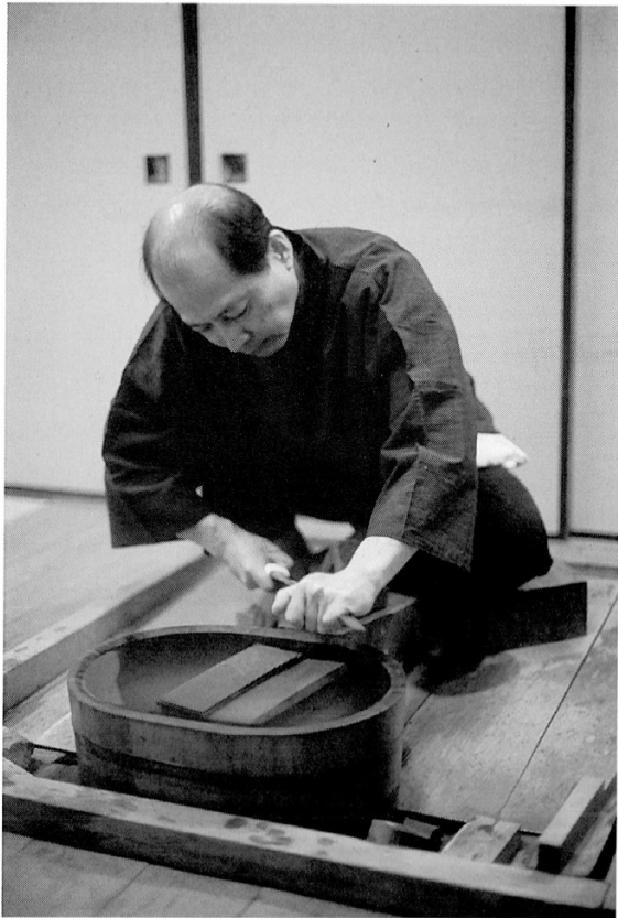
11 下地作業 (内曇砥) Shitaji process (uchigumori-to)
