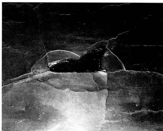
図101 塗膜割れ目の補強 Reinforcing cracks on the coating film
