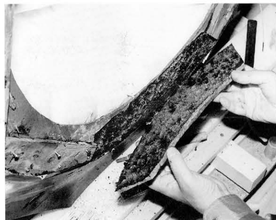
図93 麦漆で貼り付け木ネジで締めつける Using mugi-urushi and screws for fixing
