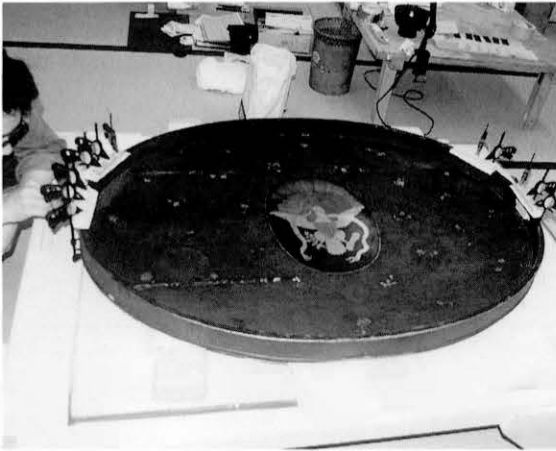
36 接着の確認 After gluing and clamping
