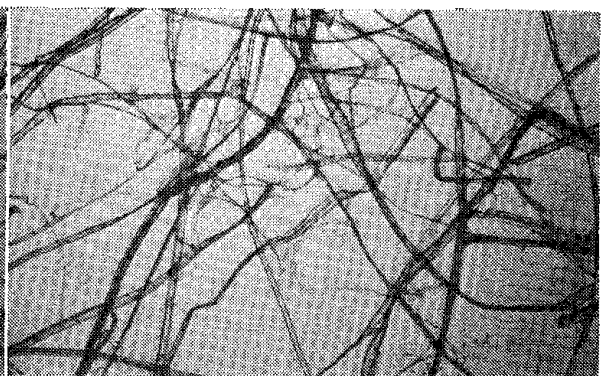
図一11 苧麻古着, 5 mm に切断, 鉄臼杵 で叩解80分間 Fig. 11 Ramie from old clothes, cut to 5 mm beaten by iron mortar and pestle 80 min.
