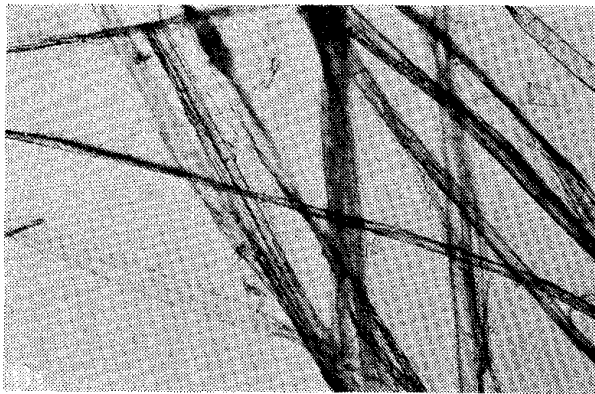
図—9 楮, 切断せずに臼杵で打解4時間 Fig. 9 Kozo, not cut, beating 4 hrs. by mortar and pestle
