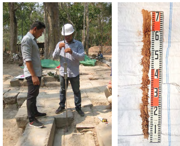
Figure 6.1.4 Implementation of the DCPT and soil sampling
