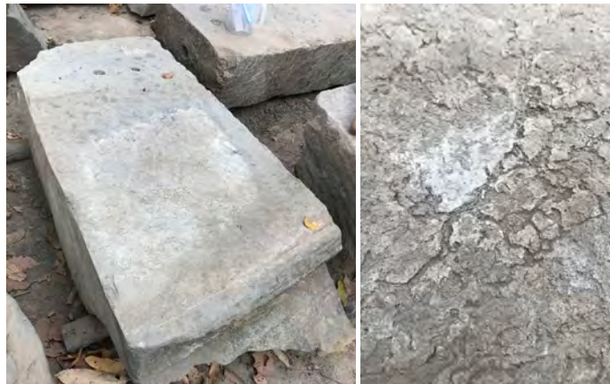
Figure 5.2.6 White substance adhered to the sandstones' upper surfaces
