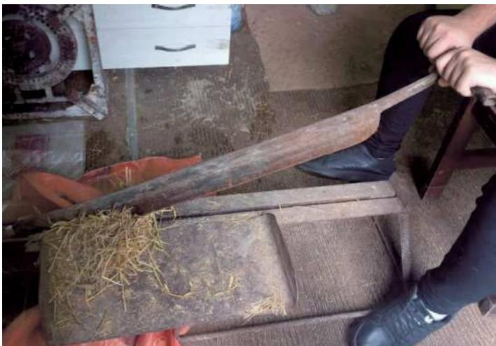
Figure 25 Cutting the fibres to pieces
