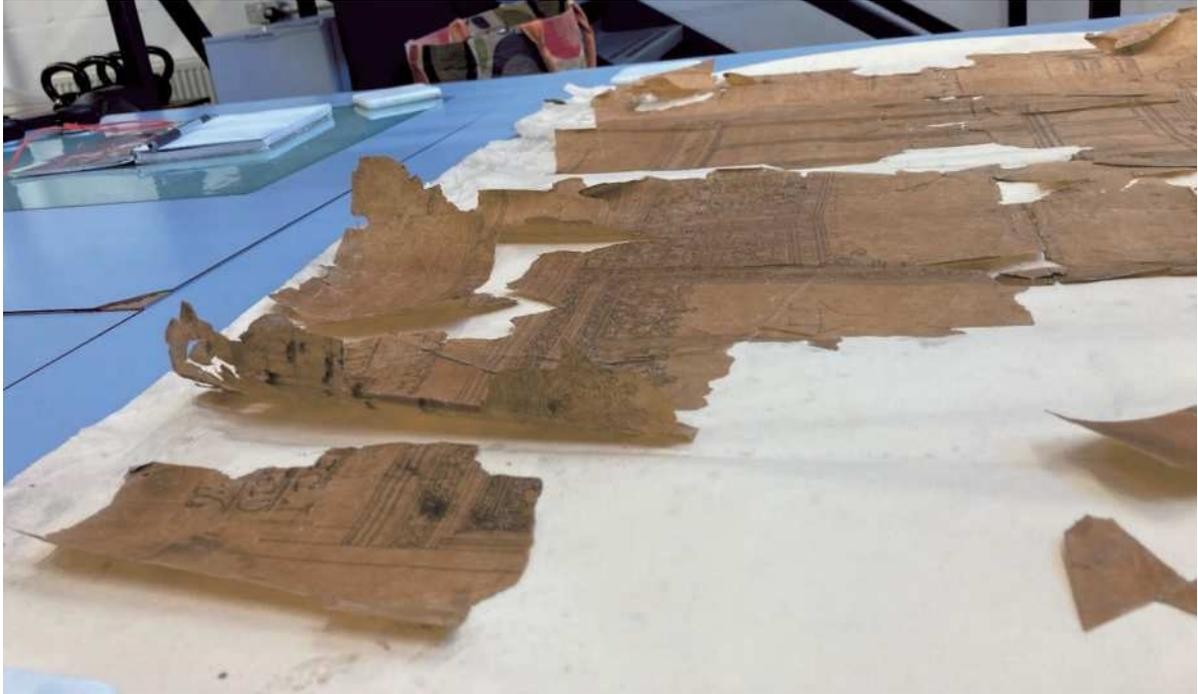
Figure 2. Detail taken before conservation treatment showing the loss of adhesive between the primary and secondary support
