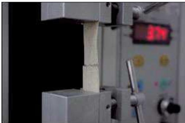
Figure 40 Measuring paper folding endurance and tensile strength
