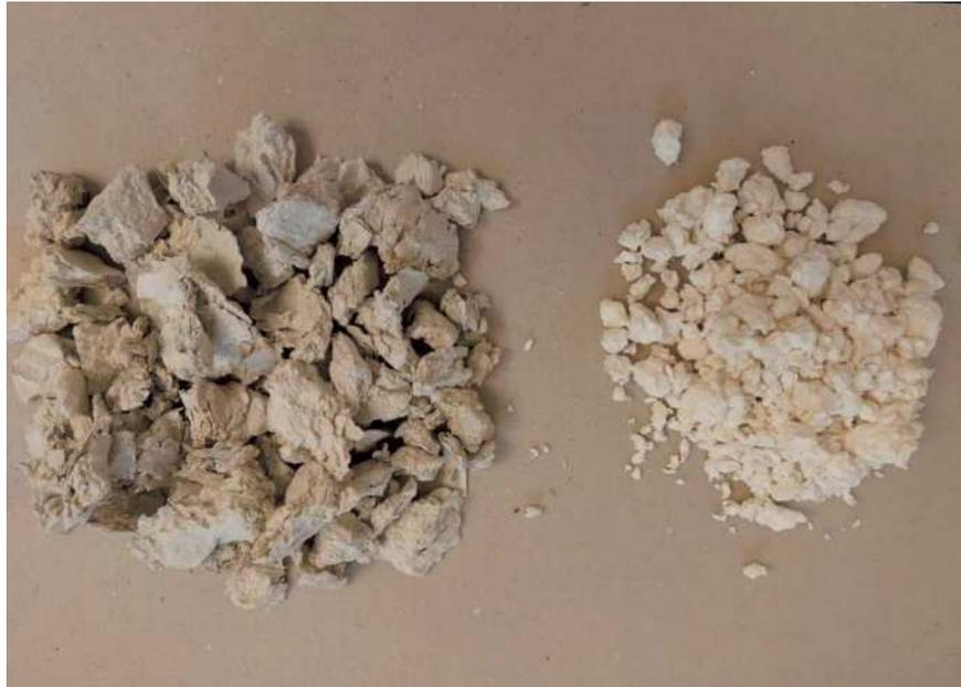
Figure 6 Inner bark are boiled with alkalis, washed and beaten to make pulp and then dried
