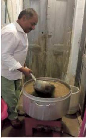
Figure 16 Boiling fibres in alkaline solution
