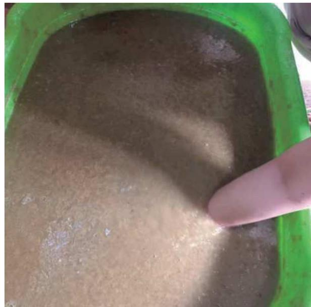
Figure 29 Adding water to paper pulp in the vat
