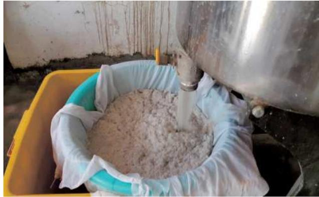
Figure 17 Washing the paper fibres thoroughly before papermaking process.
