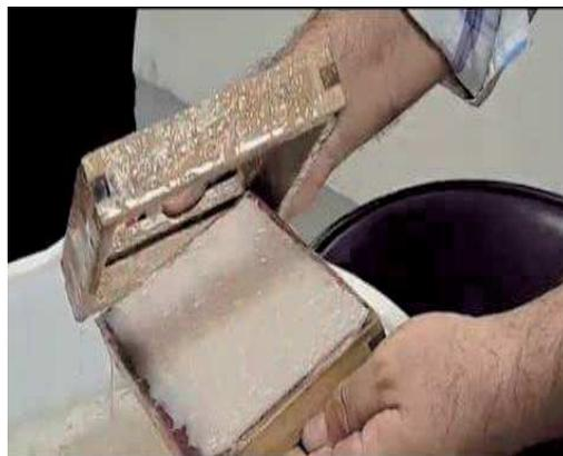
Figure 9 Formation of paper on the mold
