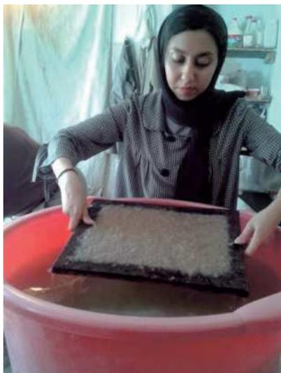
Figure 19 Formation of paper on the mold
