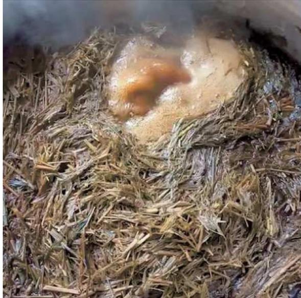
Figure 27 Boiling the fibres with alkaline solution following washing thoroughly with water
