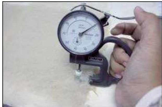
Figure 38 Measuring paper weight and thickness
