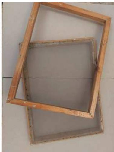
Figure 7 Wooden deckle with galvanized metal screen mold
