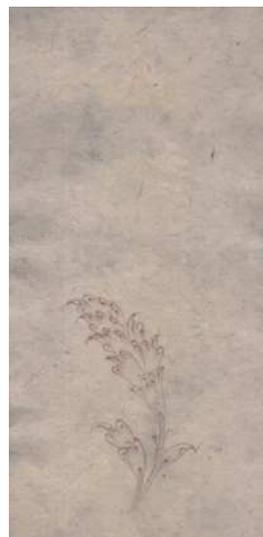
Figure 23 Paper made from hemp fibre and sized with gum arabic with gum arabic
