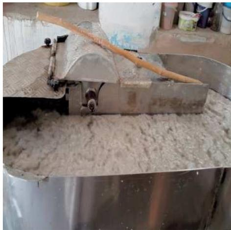
Figure 18 Using mechanical beating machine to make paper pulp
