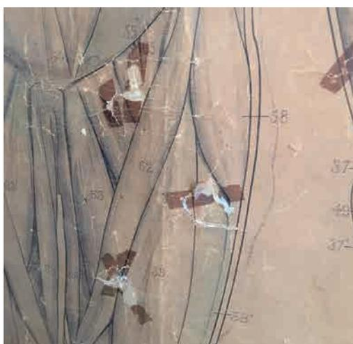
Figure 4 Damages of old pressure sensitive tapes
