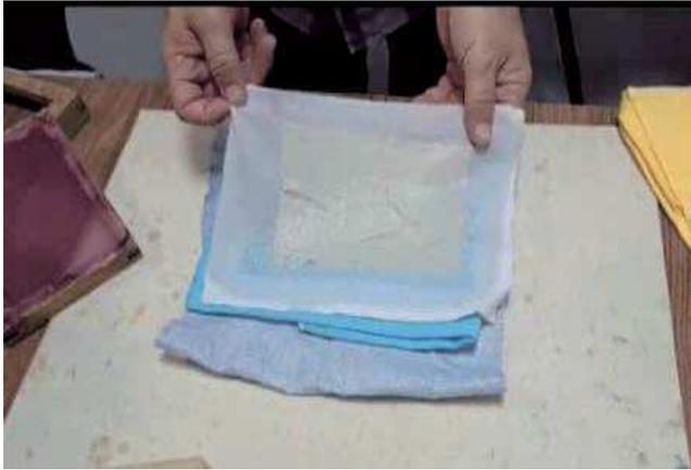
Figure 10 Transfer of paper on the cloth to press and dried
