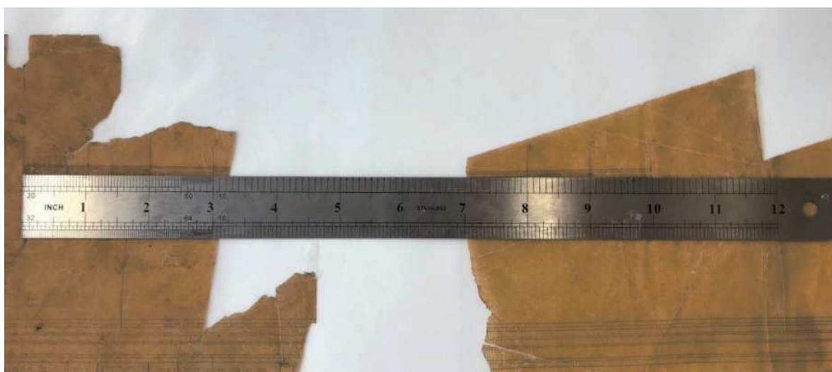
Figure 4. Using a ruler to align the scale bar on the drawing to ensure the drawing was aligned correctly
