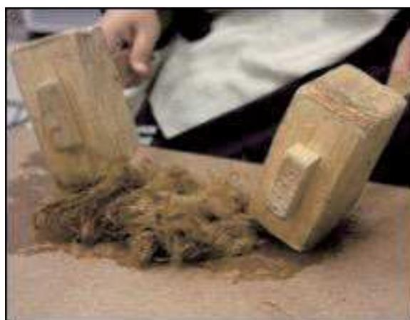
Figure 35 Beating fibre after washing thoroughly
