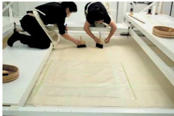
Figure 4 Using smoothing brush to backing Kozo paper
