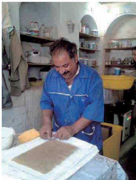
Figure 21 Each sheet of paper is separated with a layer of felt.
