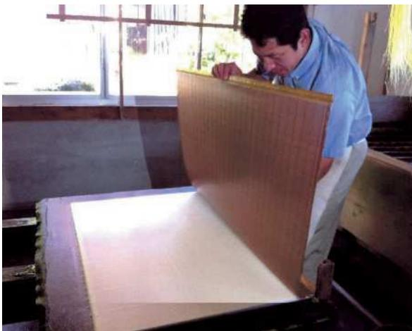
Figure 20 Laying down a sheet of *washi*, JPC 2011
