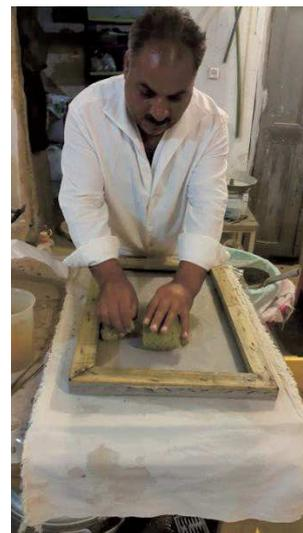
Figure 20 Transferring the paper fibre on the cloth.
