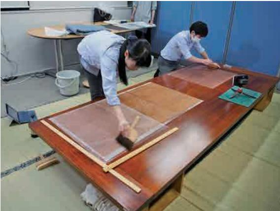
Figure 4 Smooth the surface with a *nadebake*
