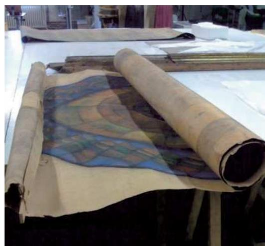
Figure 5 Mechanical damages after on a rolled preparatory cartoon.
