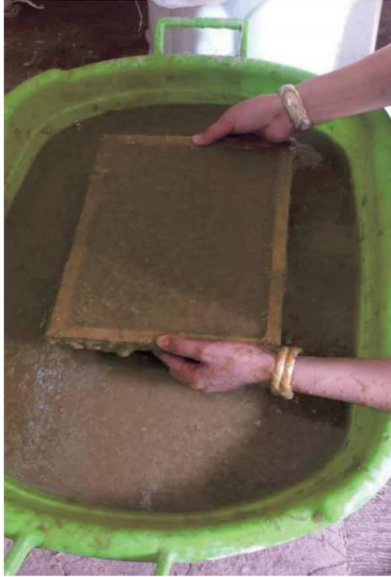
Figure 30 Formation of paper on the mold
