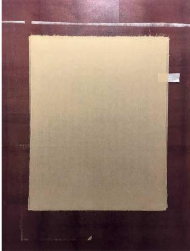
Figure 9. Two sheets of pre-toned repair paper laminated together and dried on the kari bari board
