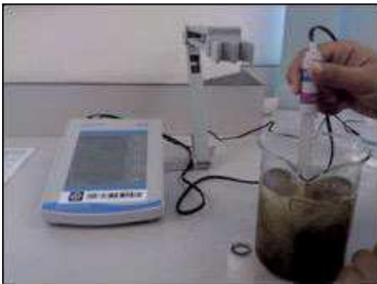
Figure 37 Measuring paper Ph test
