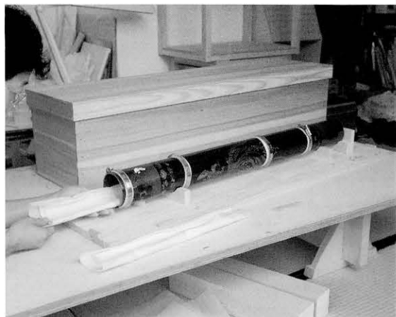
図136 加湿用の杉箱と高密度吸収スポンジ Cedar case for humidifying and highly absorbent sponge
