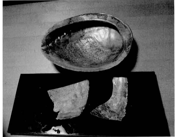
図124 孔雀鮑原貝と5日間煮立てた青貝部分 Original shell of Mexican abalone and aogai boiled for 5 days
