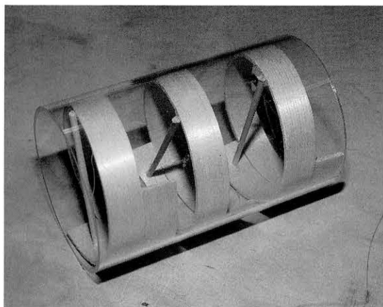
図166 アクリル製円筒と桧材 Acrylic cylinder and cypress rings
